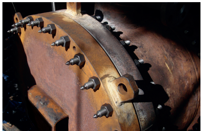
RT-Bolt load measurement underway during assembly of an exchanger channel cover with 3/4" diameter bolts
